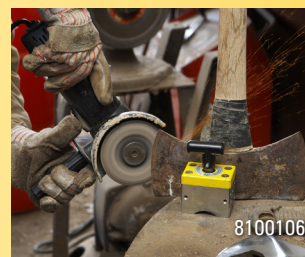
Strong hold provides make shift vise.
