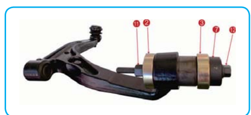
Front bushing Installation
