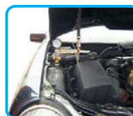
Fill new radiator liquid
