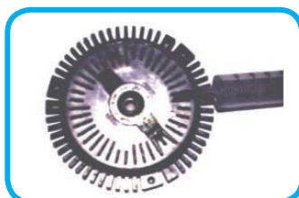
(3) Fill with the fan clutch oil. 將專用油注滿
