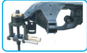
The illustration of removal of rear bush
