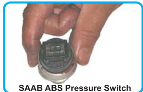
SAAB ABS Pressure Switch
