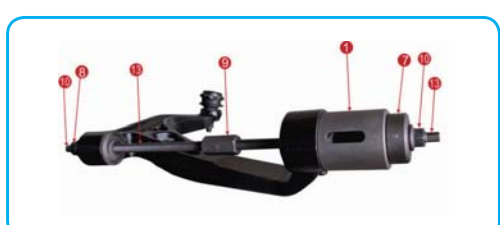
Rear bushing Extraction
