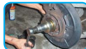
STEP 4. INSTALL BEARING
