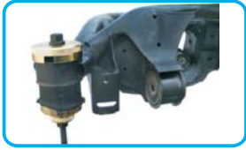
The illustration of installation of rear bush
