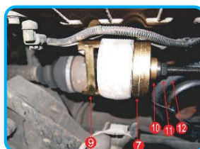
Right rear bush of engine -installation
