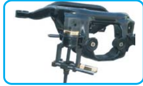
The illustration of removal of F/R bush
