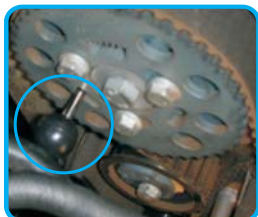
A2207-5 Injection Pump Locking Pin
