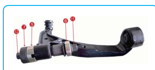
Rear bushing Installation
