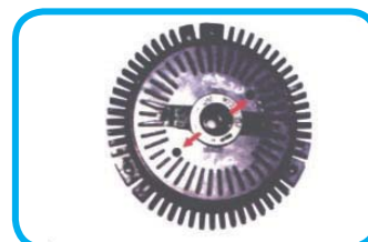
(2) Drill two small holes diameter about 2.5mm as photo. 於離合器對角線各鑽一個直徑約2.5mm的小孔
