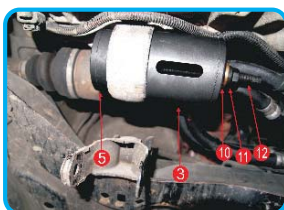
Right rear bush of engine -removal
