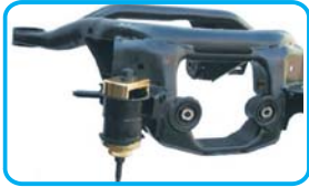
The illustration of installation of F/R bush
