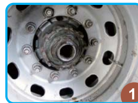
1 Firstly, Scania rear wheel nut (Dr.3/4", 8 POINTS, 100mm) should be extracted.
