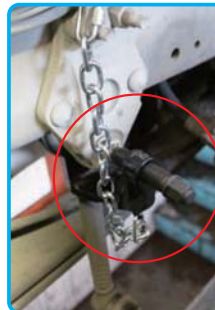
Removal of lower ball joint
