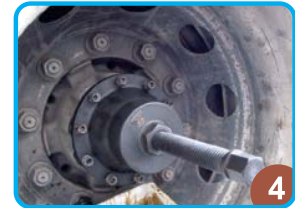
4 Finally, use A1444 with wrench to extract scania (310/320) rear wheel axle hub
