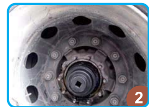
2 Use H.C.B-B1126 to extract scania rear wheel nut before using A1444
