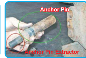
4. Anchor pin and anchor pin extractor. 來令片插銷和拔卸器示意圖。
