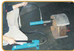
2. To remove anchor pin from brake by hydraulic hand pump. 以手動幫浦施力，將插銷由來令片中拔出。
