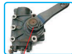
To loosen the fixed nut on the arm before using A1273
