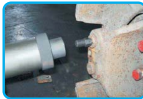
1. Connect anchor pin extractor with anchor pin and cylinder fixation. 把來令片插銷、油壓缸固定座和來令片插銷拔卸器連結。
