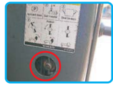
Hydraulic Valve Switch
