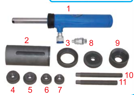
BRASS BUSH APPLICATION: SCANIA & VOLVO TRUCK
