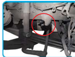
Removal of upper ball joint
